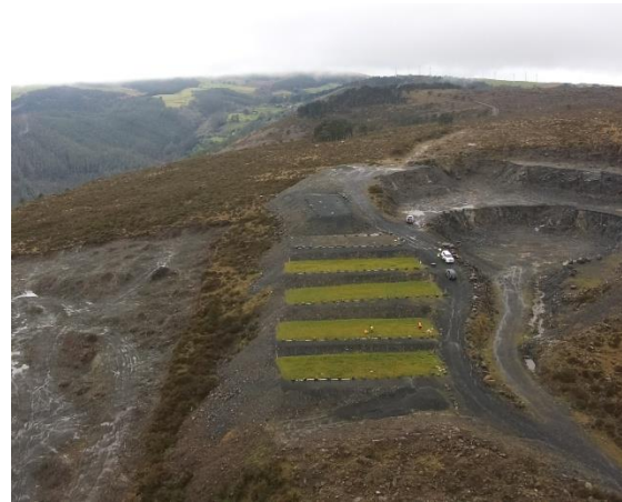
Figure 2 Aerial view of the pilot in February 2025 (4 artificial soil plots, 1 control where fertilizer was applied and trees and grasses were planted, and other second control plot that was unplanted).
