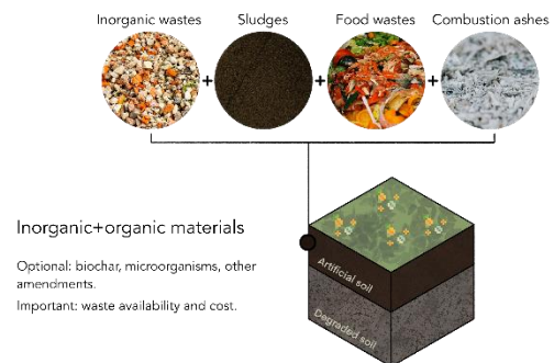
Figure 1. Diagram with examples of parent materials for artificial soil formulation
