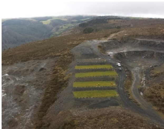
Figure 2. Aerial view of the pilot in February 2025 (4 artificial soil plots, 1 control where fertilizer was applied and trees and grasses were planted, and other second control plot that was unplanted).
